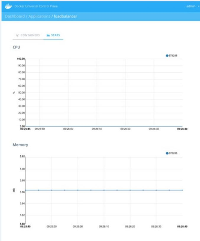
**Feature Note:** Within Docker UCP, you have the ability to monitor stats like the CPU and Memory used for the deployed applications. As well as drill down into the individual containers that make up the application.
